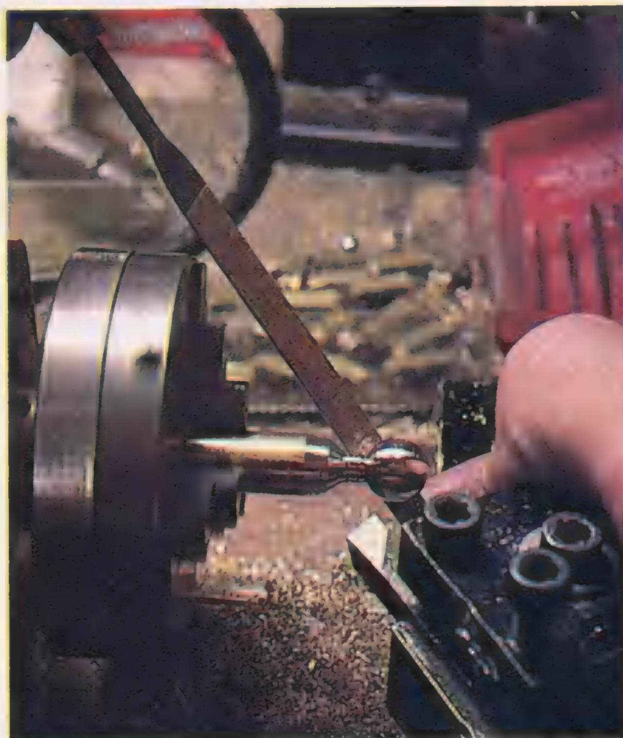
The ball is rounded off on the lathe with a file.
